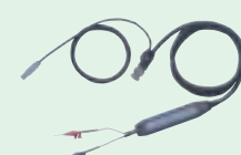
500 MHz differential probe (701920) Attenuation ratio: 1/10 with 50 Ω load Max. differential allowed voltage: ±12 V
