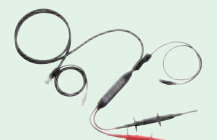
200 MHz differential probe (701922) Attenuation ratio: 1/10 with 50 Ω load Max. differential allowed voltage: ±20 V
