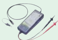
100 MHz differential probe (701924) Attenuation ratio: Can be switched between 1/100 and 1/1000 Max. differential allowed voltage: ±350 V/(1/100), ±1400 V/(1/1000)
