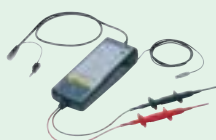
100 MHz differential probe (701921) Attenuation ratio: Can be switched between 1/10 and 1/100 Max. differential allowed voltage: ±70 V/(1/10), ±700 V/(1/100)
