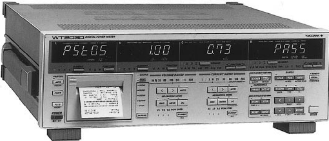
WT2030 (253103 3-phase, option added) 426 x 132 x 432 mm 10 kg (single-phase), 13 kg (3-phase, 4-wire) (16-3/4 x 5-1/4 x 17" 22.0 lbs/28.7 lbs)
